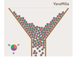
Segregation can cause poor spreading patterns, which lead to financial losses. YaraMila's hard prill, improves spreading and reduces waste. (Trials have shown that a 30% variation in spreading patterns due to segregation of poor quality blends can affect the bottom line for, for instance, winter wheat by more than 18 USD/hat)
